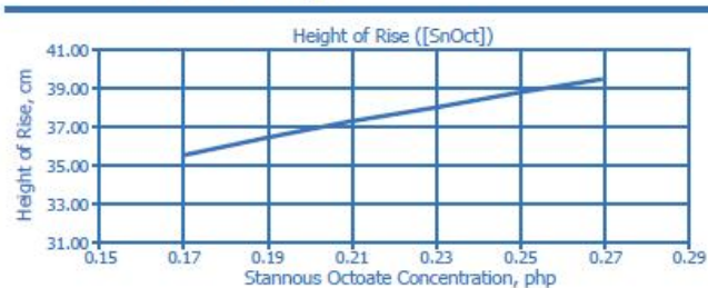
Figure 2: Effect of Tin Catalyst Concentration on Foam Height
